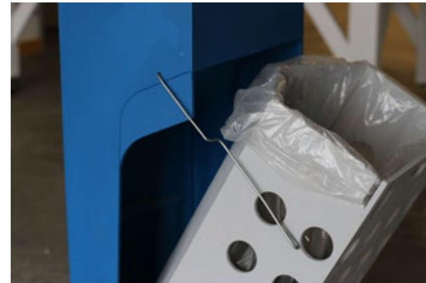
Fig. 3.3.12: Metal 'key' being used to keep the back section of the bin open.
