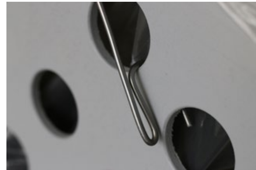
Fig. 3.3.13: Close up of the 'key' utilizing existing parts of the bin to attach to.
